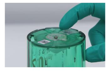
8 Re-attach the data chip to the housing by pressing it into place. Check the contact pins by running your finger over them. The pins are spring-loaded and should depress and pop back into place easily.
